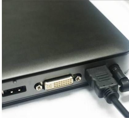
HDMI (High-Definition Multimedia Interface): This point-to-point interface is for audio and video signals designed as a single-cable solution for home theater and consumer electronics equipment.
