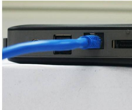
RJ-45 Connector: The connector is standard RJ-45 connector for network. Please connect to the network cable to this connector.
