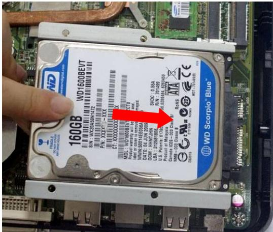
5. Fit the hard disk into HDD connector on the motherboard in this direction.
