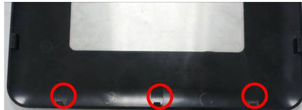
2. This edge with 3 plastic equidistant notches should be parallel to edge of the chassis' back panel.
