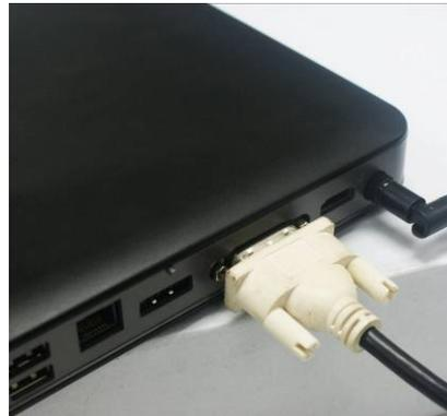
DVI (Digital Visual Interface) Connector: This interface standard designed to maximize the visual quality of digital display devices such as flat panel LCD computer displays and digital projectors.
