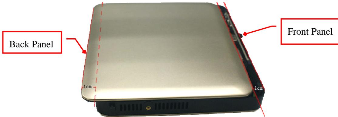
3. Place the removable cover upon the chassis. See to it that the left and right edges of the cover should be parallel to those of the chassis and there should be a distance of about 1 cm left between the front edge and the front panel of the chassis as the photo shows.
