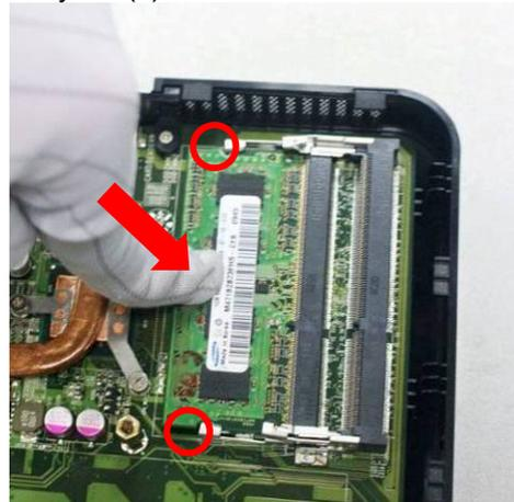
2. Insert the gold-figure side of the compatible DDRII SO-DIMM into the slot at a 30 degree.
