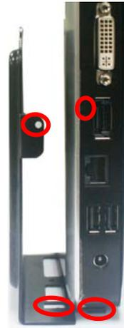
2. See to it that the square notch on the chassis is fitted into the marked square space on the stand and marked notch on the back panel of the chassis fitted in the round space of the VESA mount rack.
