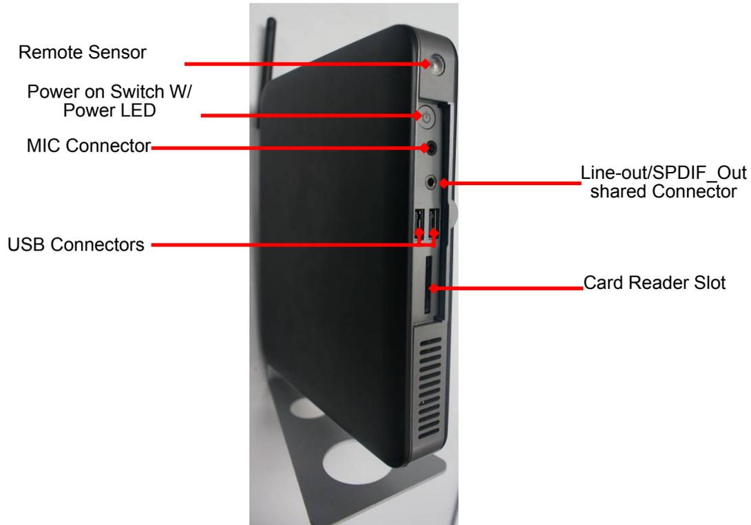
**Card Reader Slot:** to insert the MMC/SD/MS card to the front 3 in 1 card reader.
