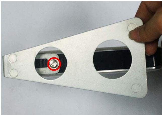
3. Lock the stand to the chassis by tightening up a screw to the marked place.
