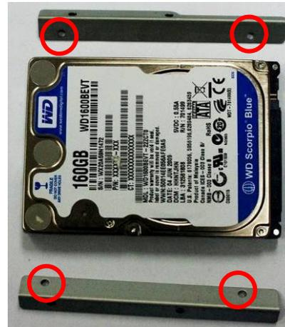
2. The SATA hard disk and the hard disk racks (see to it that the marked screw holes on rack and the corresponding holes on both edges of HDD ).
