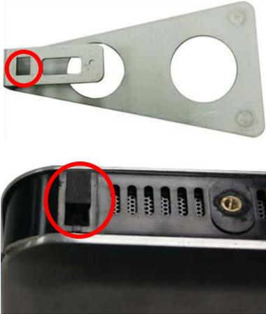
1. See to it that the marked square space fitted into the square notch on the chassis.
