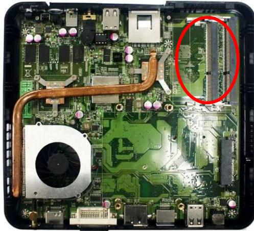
1. Locate the SO-DIMM memory slot(s) on the board.
